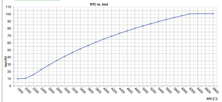
Note: Maximum dimming current is limited by NTC. NTC values, NTC High, NTC Low and NTC Minimum lout can be programmed. Using YG Programmer USB interface & YG PC based GUI Software. Default: NTC Low = 2.0K ~ 10% lout, NTC High = 6.3K, 100% lout.
